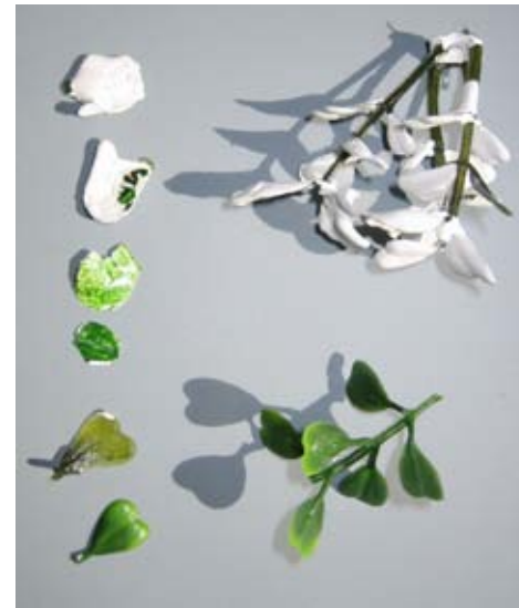
Housepaint adhered poorly to the waxy surfaces of polyethylene hedge leaves and flaked on contact. Photo: The National Museum of Denmark.
