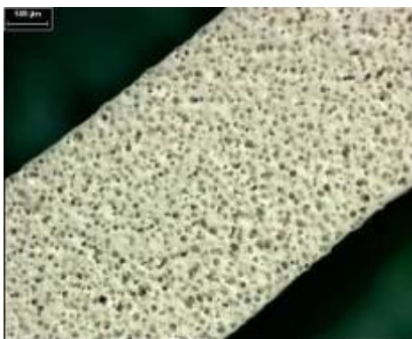
Figure 6. Using 50% recycled, micronised PVC.
