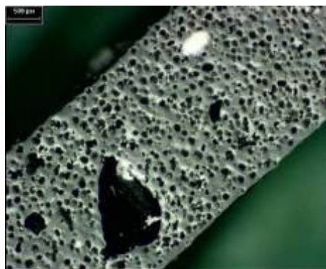
Figure 7. Using 50% recycled, milled PVC containing rubber.
